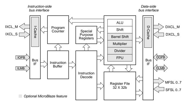
Figure 2-1: MicroBlaze Core Block Diagram
